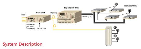
InterReach Spectrum is the leading solution for true multi-band support whether the solution supports a single service provider or multiple service providers. With it's unique flexibility and scalability, it is the best in-building wireless system for large venues and campus applications.
